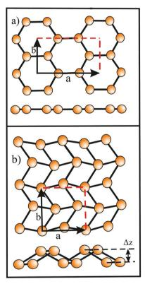
Fig. 6 (a) Honeycomb graphene-like lattice of gallenene obtained by cleaving bulk  $\alpha$ -Ga along the (100) direction after relaxation (a<sub>100</sub>-Ga). (b) Distorted rhombic lattice of gallenene obtained by cleaving bulk  $\alpha$ -Ga along the (010) direction after relaxation (b<sub>010</sub>-Ga). The dashed rectangle and square show the unit cells.
