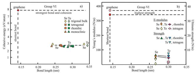
Fig. 26 (a) Plot of cohesive energies versus bond lengths of the trigonal, tetragonal, rhombic, and monoclinic phases of selenene and tellurene. (b) Young's moduli and ultimate strengths of the tetragonal and rhombic phases of selenene and tellurene as a function of bond lengths
