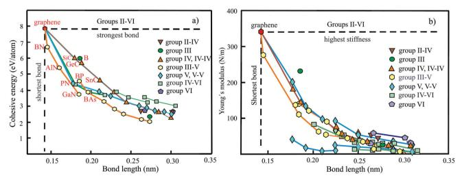
Fig. 27 (a) Overview of cohesive energies of group II-VI elemental and binary monolayers as a function of bond length. (b) Overview of the Young's moduli of group II-VI elemental and binary monolayers as a function of bond length.
