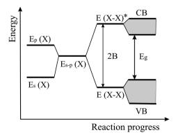
Fig. 14 Energy levels of hybridized s and p orbitals, reacting to molecular bonding and antibonding levels with level broadening and band formation of a monolaver.
