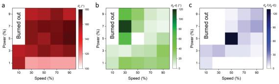
Fig. 3 Characterization of the effect of the laser speed and power settings on the surface wettability of the patterned graphene ink. (a) The advancing contact angle, (b) the contact angle hysteresis, and (c) the ratio of the advancing contact angle and the contact angle hysteresis based on the percent power vs. percent speed of the laser. Note that the groove depth and spacing are  $\sim 100 \ \mu m$  and  $\sim 250 \ \mu m$ , respectively. The drop volume is  $3 \ \mu L$ .
