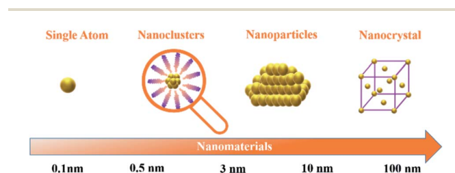
Fig. 1 Size scale from single atoms to nanocrystals.
