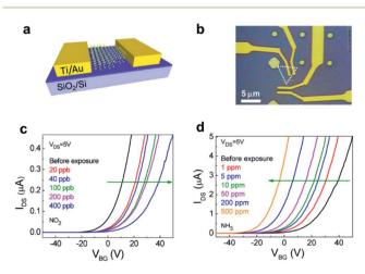
Fig. 2 (a) Schematic illustration of the MoS<sub>2</sub> FET (back-gate) as a gas sensor. (b) Optical image of two separate devices. (c and d) Transfer characteristics of the MoS<sub>2</sub> FET upon exposure to NO<sub>2</sub> and NH<sub>3</sub> of varied concentrations, respectively.50 Adapted with permission from ref. 50. Copyright 2014 American Chemical Society.
