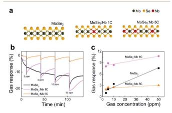
Fig. 12 (a) Schematic atomic structures of MoSe<sub>2</sub> (left), MoSe<sub>2</sub>:Nb 1C (center), and MoSe<sub>2</sub>:Nb 5C (right). (b) Transient gas response of MoSe<sub>2</sub> and doped MoSe<sub>2</sub> gas sensors to NO<sub>2</sub> concentrations varied from 3 to 50 ppm. (c) Comparison of the gas responses of the three devices versus NO<sub>2</sub> gas concentration.86 Adapted with permission from ref.86. Copyright 2017 American Chemical Society.
