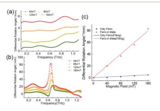
Fig. 8 Differential Faraday rotation angle spectra per mm thickness of (a) the ferromagnetic nanofluid (10.7%) in the cuvette, and (b) the ferromagnetic nanofluid in the chiral metasurface. (c) Differential Faraday rotation angle varies with the biased magnetic field at 0.65 THz for the ferromagnetic nanofluid with or without the chiral metasurface.
