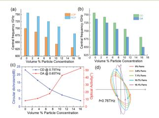
Fig. 5 (a) The shift of the central frequency of transmission spectra with the nanoparticle concentration for the LCP and RCP incidence. (b) The shift of the central frequency of CD and OA spectra with the nanoparticle concentration. (c) The CD and OA curves with the nanoparticle concentration at 0.75 THz and 0.65 THz, respectively. (d) Output polarization ellipsoid of the chiral metasurface with different ferromagnetic nanofluids for the LP incidence at 0.76 THz.
