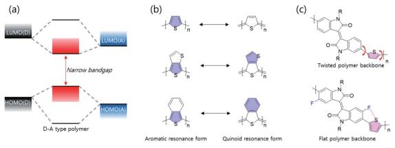
Fig. 3 Illustration of the molecular design strategies for NIR-absorbing polymer donors. (a) Band gap narrowing mechanism of a D-A type polymer. (b) Aromatic resonance form verse the quinoidal resonance form. (c) Schematic representation of the strategy for the enhancement of coplanarity along the polymer main chain.
