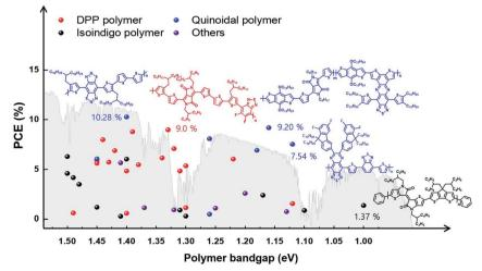
Fig. 2 Band gap and power conversion efficiency trends in narrow-band gap polymers for organic solar cells.
