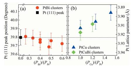
Fig. 5 Left axis: X-ray diffraction peak position of the (111) plane of the Pt fcc crystal lattice. Right axis: lattice parameter for (a) Pt clusters (black square), PtBi clusters (red circles), (b) PtCu clusters (blue triangles) and PtCuBi clusters (green diamonds). The X axis corresponds to the ratio of the powers applied on Bi or Cu magnetrons compared to the power on the Pt magnetron  $(P_x/P_{\rm Pt})$  with  $x={\rm Bi}$ , Cu.
