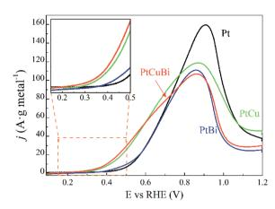
Fig. 9 Polarization curves for the oxidation of 0.10 mol L $^{-1}$  glycerol recorded for Pt/C (black line), PtBi/C (blue line), PtCu/C (green line) and PtCuBi/C (red line) materials ( $v=0.005\,\mathrm{V}\,\mathrm{s}^{-1}$ , N $_2$ -saturated 0.10 M NaOH electrolyte,  $T=20\,\mathrm{°C}$ ). Inset: zoomed-in image of the oxidation potential onset region.
