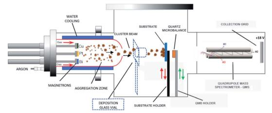
Fig. 1 Schematic of the adjustable multimagnetron based GAS used for the multimetallic cluster synthesis, adapted from a Mantis Nanogen 50 system.
