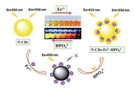
Scheme 1 Schematic illustration of the N-CDs as a nanosensor for the detection of  ${\rm Fe}^{3+}$  and  ${\rm HPO_4}^{2-}$  with obvious "on–off–on" fluorescence behaviour in aqueous solution.
