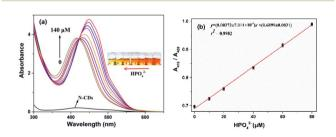
Fig. 5 (a) Absorption spectra of the N-CDs-Fe<sup>3+</sup> complex in pure water with the different concentrations of  $HPO_4^{\ 2-}$  (0-140  $\mu M$ ). The inset is the image of the N-CDs-Fe<sup>3+</sup> complex in pure water with the increased HPO<sub>4</sub><sup>2-</sup> from right to left under daylight. (b) Linear relationship between ratiometric absorbance  $(A_{415}/A_{450})$  and the concentration of  $HPO_4^{2-}$ .
