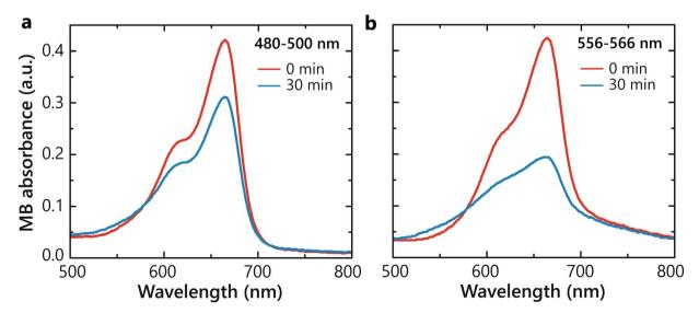
Fig. 4 The effect of the illumination wavelength. MB absorbance spectra before and after 30 min photocatalytic degradation in water with SiO<sub>2</sub>-Au<sub>(3)</sub>-Pt<sub>+++</sub> hetero-nanoparticles under the illumination in the spectral range of (a) 480-500 nm and (b) 556-566 nm with the same average absorbed power.
