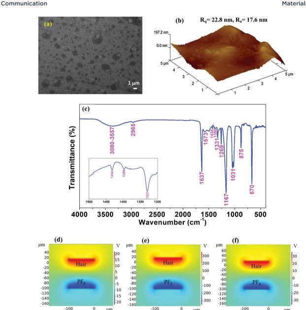
Fig. 3 (a) FESEM view of the human hair-based film. (b) AFM image (three-dimensional) of the human hair-based film. (c) FTIR spectra of the human hair-based film with an expanded spectrum view of a certain region  $(1300-1500 \text{ cm}^{-1})$  in the inset. COMSOL simulation results of the TENGs comprising the human hair based film and (d) PF<sub>0</sub>, (e) PF<sub>2</sub>, and (f) PF<sub>4</sub> film.
