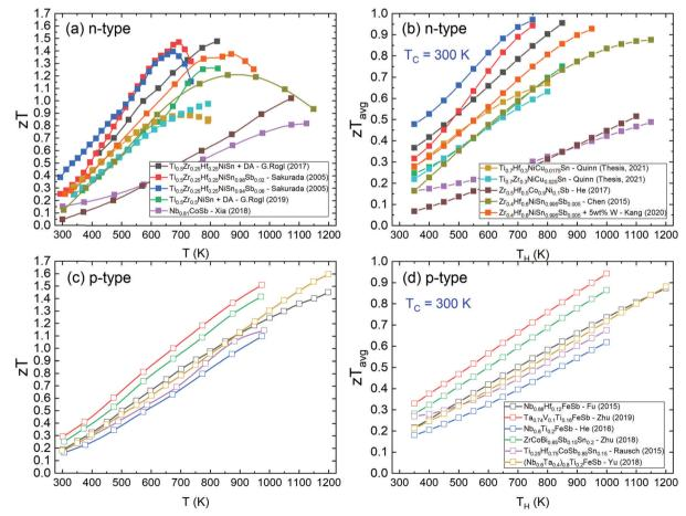
Fig. 4 Literature zT values of the best n-type and p-type half-Heusler thermoelectric materials. Panels (a) and (b) show zT and the average  $zT_{avg}$  of n-type samples as a function of temperature. Panels (c) and (d) show zT and the average  $zT_{avg}$  of p-type samples. XNiSn systems have large low temperature zT, but their increase slows above 800 K due to onset of bipolar transport linked to the relatively small band gap.
