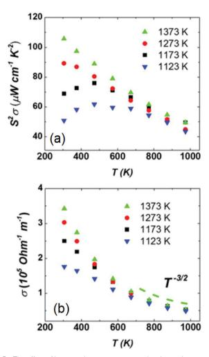
Fig. 5 The effect of hot-pressing temperature on the electronic properties of Nb<sub>0.95</sub>Ti<sub>0.05</sub>FeSb. As seen in (a) hot-pressing at 1100 °C leads to over double the power factor,  $S^2\sigma$  at 300 K, relative to pressing at 950 °C. As illustrated in (b) this enhancement arises due to an increase in  $\sigma_{300K}$ attributed to the elimination of grain boundary scattering of charge carriers. Reproduced from He et al. PNAS, 2016.99
