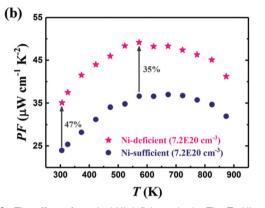
Fig. 6 The effect of nominal Ni deficiency in the Ti<sub>1-x</sub>Ta<sub>x</sub>Ni<sub>1-a</sub>Sn system, in samples with identical carrier concentration,  $n_{\rm H}$ . As seen in (a), nominal Ni deficiency causes a substantial increase in  $\mu_H$  at 300 K and enhances S(T) at high temperatures. This leads to a significant increase in power factor,  $S^2\sigma$  as seen in (b). Reproduced from Ren et al. 2019, Advanced Electronic Materials.71
