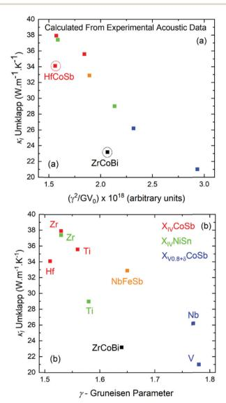
Fig. 3 Plots of calculated lattice thermal conductivity ( $\kappa_{\rm l}$ ) at 300 K (see Section 2.4), assuming the presence of only Umklapp scattering (i.e. for the defect free parent materials), versus (a) the variables determining the magnitude of Umklapp scattering and (b) the acoustic Grüneisen parameter. HfCoSb and ZrCoBi have lower  $\kappa_l$  due to low  $v_s$  (see Table 2).
