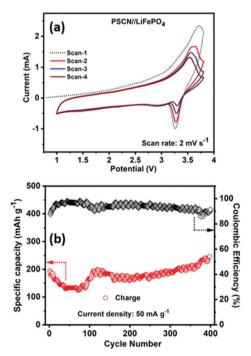
Fig. 6 Full cell LIB performance of a PSCN anode coupled with a LiFePO<sub>4</sub> cathode. (a) Cyclic voltammetry profiles at a scan rate of 2 mV  $\rm s^{-1}$  at 1.0 – 3.6 V, and (b) cycling performance and the corresponding coulombic efficiencies at 50 mA g<sup>-1</sup> of current density.
