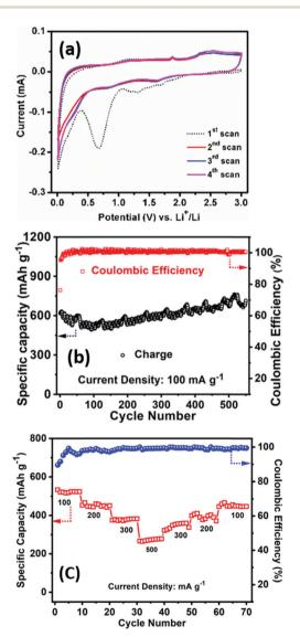
Fig. 5 Electrochemical half-cell LIB anode performance of the PSCNs. (a) Cyclic voltammetry of the PSCN electrode for the first four cycles at 0.1 mV  $s^{-1}$  at 0.01–3.0 V, (b) cycling performance at 100 mA  $g^{-1}$ current density, and (c) rate performance at different current densities  $(100-500 \text{ mA g}^{-1})$
