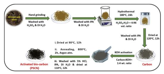
Scheme 1 Schematic representation for the synthesis of activated N,S-doped spherical porous carbon nanostructures (PSCN)
