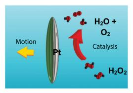
Fig. 1 Schematic of an ellipsoidal micro swimmer, coated along its major axis with platinum (shaded grey) decomposing hydrogen peroxide fuel.
