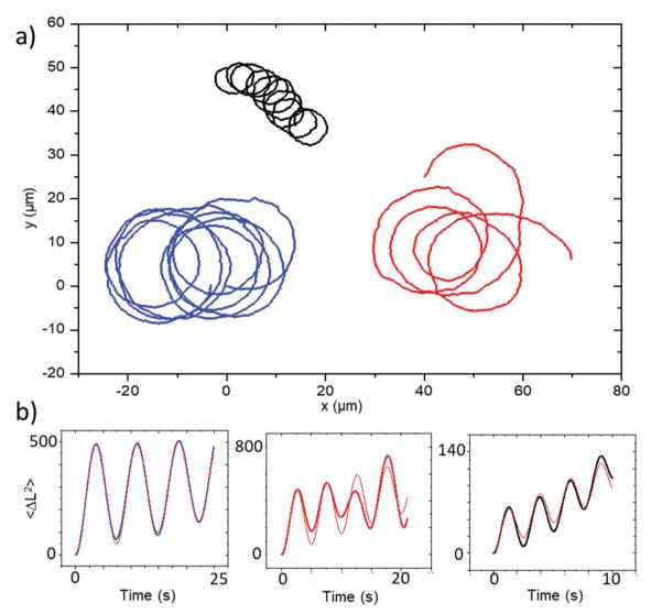
Fig. 7 (a) Trajectories and (b) corresponding MSD plots representative of the batch of Janus ellipsoids coated at a glancing angle of 60°. MSD fitting plots are shown in red.
