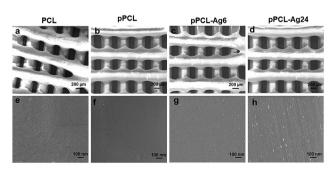
**Fig. 2** SEM images of PCL, pPCL–Ag6, and pPCL–Ag24 at (a–d) lower and (e–h) higher magnifications.
