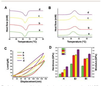
Fig. 4 Assessment of the thermal and mechanical properties of (a) PCL, (b) pPCL, (c) pPCL-Ag6 and (d) pPCL-Ag24 from the (A) DSC melting thermogram, (B) DSC crystallization thermogram, (C) nanoindentation load-displacement curves at a peak displacement of 150 nm and (D) comparison of hardness (H), reduced modulus (Er) and modulus of elasticity (Et).
