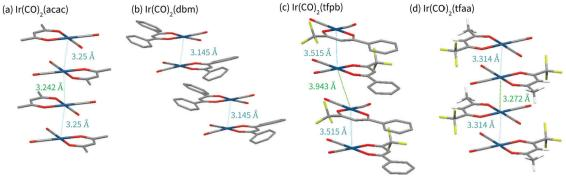
Fig. 3 Schematic of the crystal structures of (a) Ir(CO)<sub>2</sub>acac, (b) Ir(CO)<sub>2</sub>tfpb, (d)Ir(CO)<sub>2</sub>tfpb, (d)Ir(CO)<sub>2</sub>tfaa, obtained via single-crystal X-ray diffraction. Note that (b) and (c) have two molecules in each asymmetric unit. For all complexes, four molecules are shown to illustrate packing along the axis perpendicular to the plane of the molecules.
