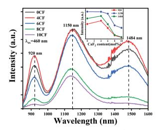
Fig. 1 The emission spectra ( $\lambda_{\rm ex}$  = 460 nm) of the xCF (x = 0, 4, 6, 8, and 10) glass samples. The inset is the integral intensity of the ~920, ~1150, and ~1484 nm emission bands as a function of the content of fluoride.
