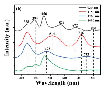
Fig. 4 Excitation spectra at 930, 1150, 1260 and 1490 nm for the BF sample.
