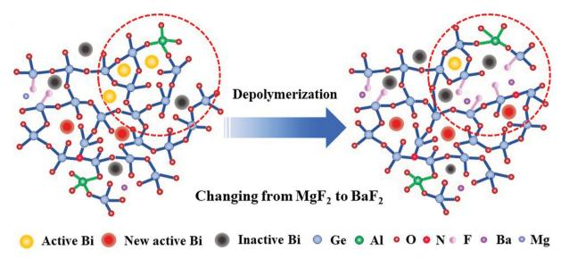
Evolution of the microscopic structure of the glasses MF to BF.
