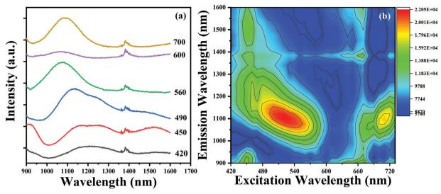
Fig. 7 (a) The NIR spectra evolution of the BF glass sample. (b) The contour plot of the emission-excitation map from the BF glass sample.
