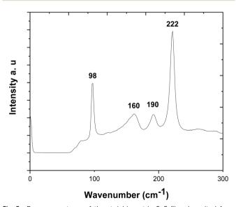
Fig. 5 Raman spectrum of the stoichiometric SnS film deposited from precursor (2) with the data highlighting the  $A_g$  (98, 190, 222 cm<sup>-1</sup>) and  $B_{3g}$ (160 cm<sup>-1</sup>) modes.
