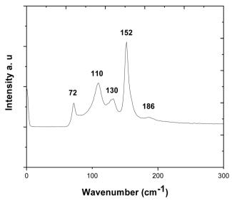
Fig. 8 Raman spectrum collected for an SnSe thin film with the peaks at 152, 130 and 110 cm $^{-1}$ , corresponding to the  $A_{3q}$ ,  $A_{2q}$  and  $B_{3q}$  modes.
