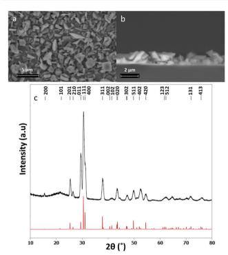
Fig. 6 (a) Top down SEM image of an SnSe deposit, (b) cross sectional SEM image of the same film showing a film thickness of ca. 1.3  $\mu m$  and (c) grazing incidence XRD pattern for SnSe thin film (black) and the pattern for bulk Pnma SnSe (red).53
