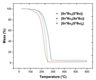
Fig. 1 TGA profiles for (1) (green), (2) (blue) and (3) (red). The TGA experiments were conducted with a temperature ramp rate of 5  $^{\circ}$ C min $^{-1}$  and a constant flow of argon gas at a flow rate of 30 mL min $^{-1}$ .
