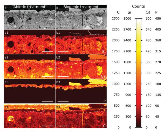
Fig. 5 A selection of the EPMA-WDS maps of the abiotic sample (a) and the biogenic sample (b); a and b are the backscatter electron images, (a1-a4 and b1-b4) are the elemental maps (WDS) for Si (a1 and b1), Ca (a2 and b2), P (a3 and b3), and C (a4 and b4). The dashed lines demarcate surface layers within the cement blocks with a high P signal; the dash dotted lines outline large areas on top of the cement layers with a high P and high Ca signal. The scale bar represents 100 µm.
