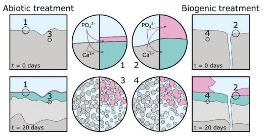
Fig. 8 Schematic representation of a proposed conceptual model; grey represents the unaltered cement, light grey represents altered cement where calcium rich phases dissolved, pink represents hydroxyapatite phases and green represents cement phases intermixed with hydroxyapatite phases.
