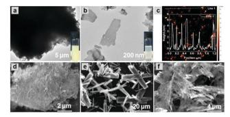
Fig. 1 TEM images of (a) bulk  $g-C_3N_4$  and (b) CNNS exfoliated using scCO<sub>2</sub>/CTAB. (c) AFM image of CNNS, inset: height of the CNNS as determined by AFM; SEM images of (d) bulk q-C<sub>3</sub>N<sub>4</sub>, (e) MFM-300(Fe), and (f) CNNS/MFM-300(Fe) composite. The composites shown here all have a g-C<sub>3</sub>N<sub>4</sub>: MOF wt: wt ratio of 7:3
