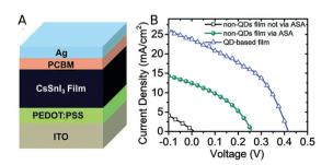
Fig. 3 (A) Device structure of the solar cell based on the CsSnI<sub>3</sub> films. (B) J-V curves of CsSnI<sub>3</sub> bulk solar cell (black), CsSnI<sub>3</sub> bulk solar cell with the addition of TPPi as antioxidant additive (green) and CsSnI<sub>3</sub> NCs solar cell with TPPi (blue). Reproduced from ref. 58 with permission from the Royal Society of Chemistry (RSC, Journal of Materials Chemistry A).
