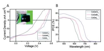
Fig. 4 (A) J-V characteristics of CsGel<sub>3</sub> (blue), CsGeBr<sub>3</sub> (red), and CsGeCl<sub>3</sub> (black) solar cells. The inset shows a picture of a solar cell. (B) Incident Photon-to-electron Conversion Efficiency (IPCE) of CsGeX<sub>3</sub> perovskite devices with different halides. Reproduced from ref. 80 with permission from the Royal Society of Chemistry. (RSC, RSC Advances).
