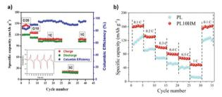
Fig. 11 Rate performance of a Li/Mg-BTC/LiFePO<sub>4</sub> hot pressed cell at 70 °C and corresponding cycling profile<sup>142</sup> (a); rate performance of the PEO/HKUST-1 SPE at 50 °C when compared with a PEO SPE (b). 136
