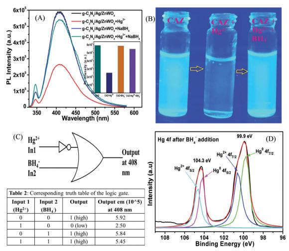
Fig. 9 (A) PL effect of NaBH<sub>4</sub> on g-C<sub>3</sub>N<sub>4</sub>/Ag/ZnWO<sub>4</sub>-Hg<sup>2+</sup>. (B) Photographic image of experiment (A) under 365 nm light. (C) Implication logic gate obtained from the results of (A) and (D) X-ray photoelectron spectroscopy of Hg 4f after the addition of  $\mathrm{BH_4}^-$
