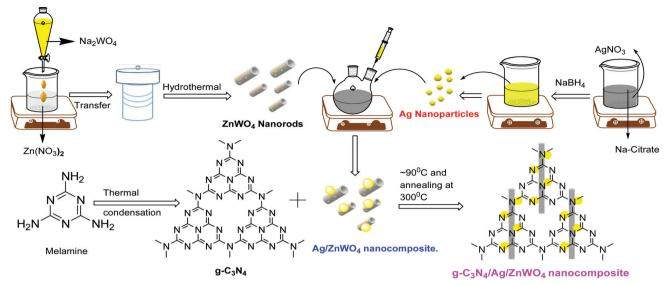
Scheme 1 Proposed synthetic scheme to prepare g-C<sub>3</sub>N<sub>4</sub>/Ag/ZnWO<sub>4</sub> nanocomposites
