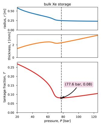
Fig. 3 Optimizing the compressed, bulk xenon storage system at 298 K. The radius of the vessel, the thickness of its walls, and the tankage fraction are shown as a function of the storage pressure. The optimal storage pressure (vertical, dashed line) minimizes the tankage fraction.
