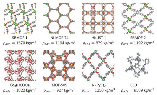
Fig. 4 The crystal structures of the nanoporous material candidates we consider for adsorbed xenon propellant storage and their (crystal) densities, ρ<sub>ads</sub> For CC3, a molecular material, we show only a single cage.
