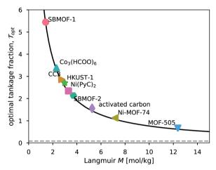
Fig. 7 The relationship between the tankage fraction of each optimized adsorbed xenon storage system and the saturation loading of xenon in the adsorbent, M. The solid curve shows the approximation to the optimal tankage fraction in egn (13)
