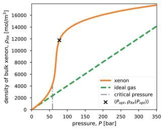
Fig. 2 The density of xenon,  $\rho_{Xe} = \rho_{Xe}(P)$ , as a function of pressure, P, at a fixed temperature of 298 K, taken from NIST.  $^{26}$  For comparison, the density of the ideal gas is also shown. The vertical, dashed line marks the critical pressure of xenon ( $P_c$  = 58.42 bar. Note  $T_c$  = 289.74 K.). The x marks the optimal storage conditions in a bulk xenon propellant storage system, which we will derive later.
