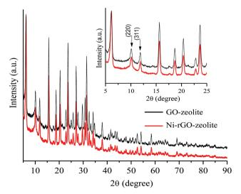
Fig. 3 XRD patterns of GO-zeolite and Ni-rGO-zeolite composites.
