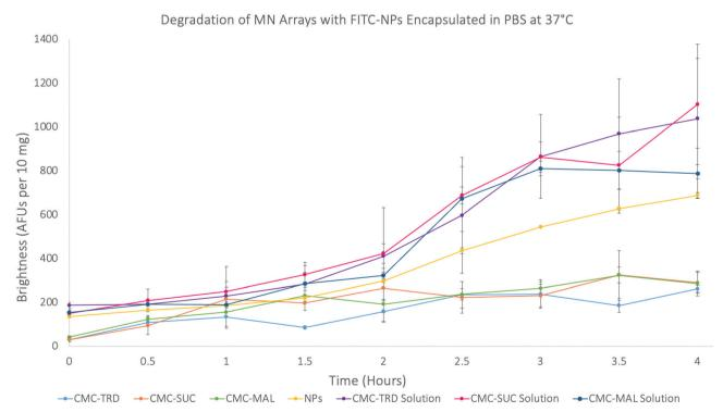
Fig. 6 Graph showing the degradation of microneedle arrays with FITC-SiNP encapsulated at 37 °C over 4 hours.
