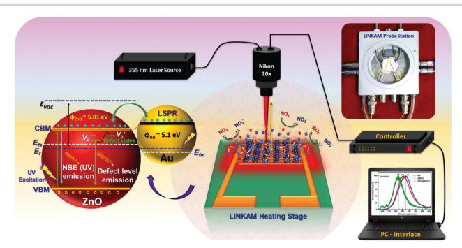
Scheme 1 Schematic depiction of experimental set up used for operando photoluminescence studies performed for ZnO-GNI HNFs upon NO2 exposure
