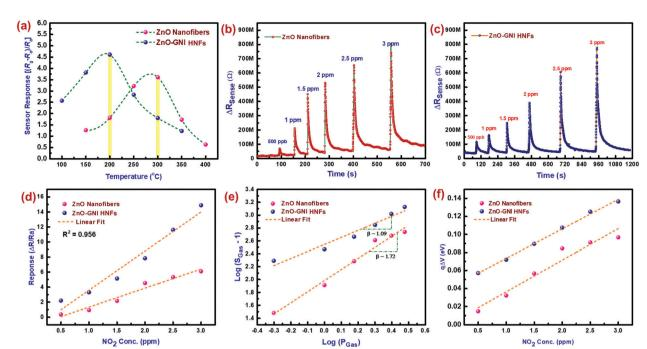
Fig. 6 (a) Sensor response graph of NO<sub>2</sub> versus different temperature, (b and c) NO<sub>2</sub> sensor response-recovery plots of pristine ZnO and aligned heterojunction ZnO-GNI HNFs at its operational temperature, (d) sensor response against NO<sub>2</sub> concentration, (e)  $\log(S_{\rm qas}-1)$  versus  $\log(P_{\rm qas})$  plot toward 0.5-3 ppm of NO<sub>2</sub> gas and (f) effect of band bending upon increasing NO<sub>2</sub> concentration
