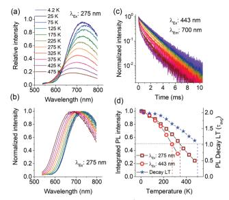
Fig. 4 Temperature dependent PL of Mn<sup>2+</sup> (10 at%) doped Ca- $\alpha$ -SiAlON under 275 nm excitation (a); PL in normalized scale (b); PL decay curves (c); and the plot of integrated PL intensity (under 275 nm and 443 nm excitations) and the PL decay time with temperature (d). In (a), (b) and (c), the line colors are as indexed in (a). In (d), the integrated PL values were derived from 535-800 nm spectral range.
