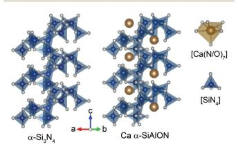
Fig. 1 Crystal structure of  $\alpha$ -Si $_3$ N $_4$  and Ca- $\alpha$ -SiAlON along c-axis. The brown, blue and gray spheres represent Ca, Si/Al, and N/O ions, respectively. The coordination polyhedron of Ca and Si tetrahedron are presented in right side.
