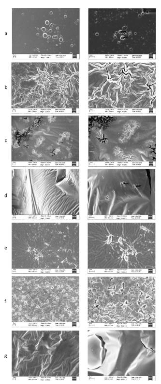
Fig. 8 SEM images of the (a) F/AA, (b) F/Tween, (c) F/bet:LA NaDES, (d) F/ChCl:LA NaDES, (e) F/0.5LA (f) F/bet:LA mix. and (g) F/ChCl:LA mix. Images on the left are at 5  $\times$   $10^3\times$  magnification and on the right at  $10^4\times$  magnification.
