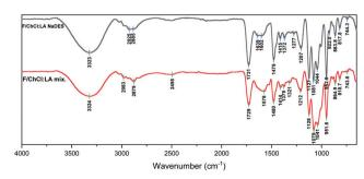
Fig. 7 FT-IR spectra of the F/ChCl:LA NaDES (top) and the F/ChCl:LA mix. (bottom).
