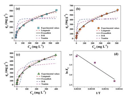
Fig. 6 Experimental data fitted in the Langmuir, Freundlich, D–R, Temkin isotherm model for  $Cr(v_1)$  adsorption on the **PPY–PANI@RHA** nanocomposite at (a) 293 K, (b) 303 K, and (c) 313 K temperatures. (d) Van't Hoff plot of  $lnK_C$  versus 1/T for  $Cr(v_1)$  adsorption on **PPY–PANI@RHA** at a constant adsorbent dose of 0.8 g  $L^{-1}$  and pH 2.
