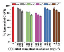
Fig. 7 Effect of co-existing (a) cations, (b) anions on the removal of  $Cr(v_1)$  by **PPY-PANI@RHA**. (Initial  $Cr(v_1)$  concentration: 50 mg  $L^{-1}$ ; contact time: 300 min; agitation speed: 200 rpm; pH  $\sim$  2; temperature: 303 K).
