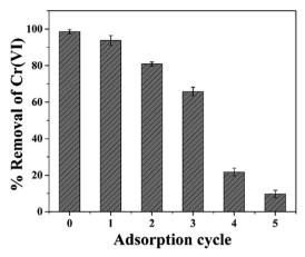
Fig. 9 Reusability capacity of PPY-PANI@RHA up to five cycles for the removal of  $Cr(v_i)$  (Initial  $Cr(v_i)$  concentration: 50 mg  $L^{-1}$ ; regenerated PPY-PANI@RHA dose: 0.8 g L<sup>-1</sup>; contact time: 300 min; agitation speed: 200 rpm; pH ~ 2; temperature: 303 K).
