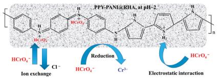
Fig. 8 Schematic representation of possible Cr(vi) adsorption by PPY-PANI@RHA
