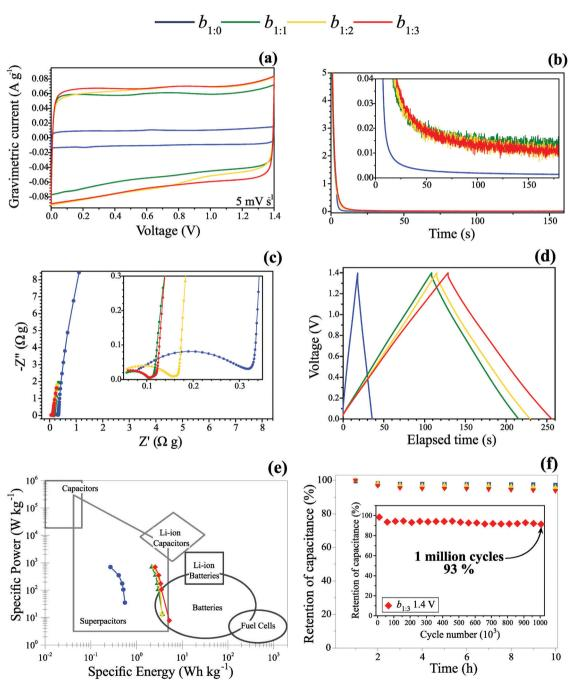
Fig. 5 Electrochemical data and performance of the symmetric coin cell as a function of the MWCNT: AC mass ratio: (a) cyclic voltammograms at  $5 \text{ mV s}^{-1}$ , (b) transient currents during the SSC experiments at 1.4 V, (c) EIS at 1.4 V, (d) GCD at  $0.15 \text{ A g}^{-1}$ , (e) the Ragone plot, and (f) capacitance retention after 1 million cycles. Electrolyte: 1.0 mol dm<sup>-3</sup> Li<sub>2</sub>SO<sub>4</sub>.
