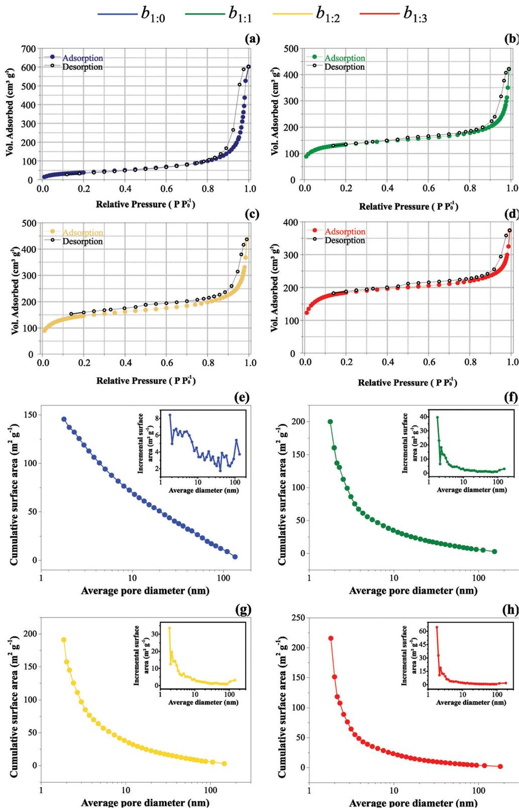
Fig. 4 (a–d) Nitrogen isotherms and (e–h) pore size distribution obtained for the different carbon-based samples used in the BET analysis: (a and e)  $b_{1:0}$ , (b and f)  $b_{1:1}$ , (c and g)  $b_{1:2}$ , and (d and h)  $b_{1:3}$ .
