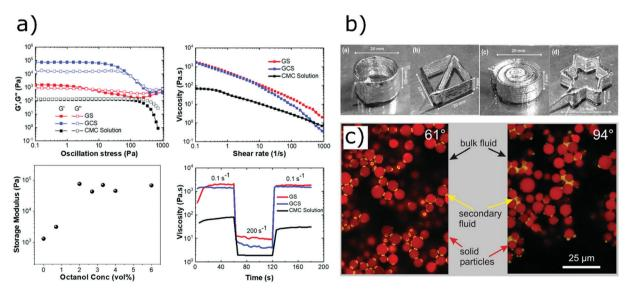
Fig. 14 (a) Rheological properties of capillary suspensions before and after the addition of the secondary fluid (adapted with permission from ref. 143, Published by The Royal Society of Chemistry); (b) 3D printed liquid metal inks (adapted with permission from ref. 144, Copyright 2018 John Wiley and Sons); (c) secondary fluid linking the solid particles of a capillary suspension (adapted with permission from ref. 140, Copyright 2016 American Chemical Society)
