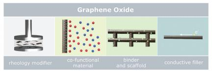
Fig. 11 Schematics showing the functions fulfilled by graphene oxide in DIW inks.
