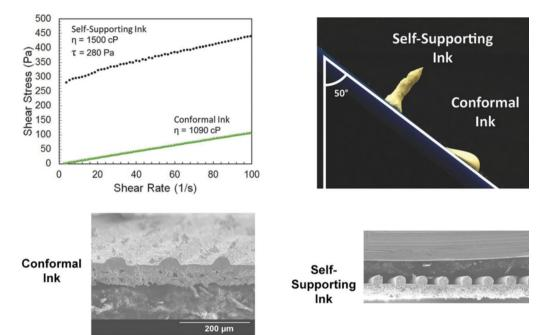
Fig. 16 Comparison between the self-supporting and conformal inks formulated by McOwen *et al.*<sup>90</sup> (adapted with permission from ref. 90, Copyright 2018 John Wiley and Sons).
