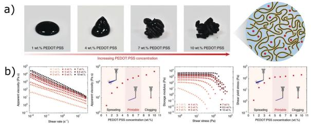
Fig. 13 (a) Images of the PEDTO: PSS inks at different polymer concentrations and schematic showing the network of entangled nanofibers in the inks; (b) rheology of PEDOT:PSS inks at different concentrations (all panels adapted with permission from ref. 138, Copyright 2020 Springer Nature).
