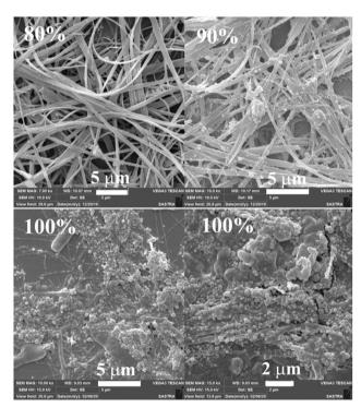
Fig. 4 SEM images of 3 at different water fractions in a  $CH_3CN$ -water mixture (scale bar = 1  $\mu$ m).
