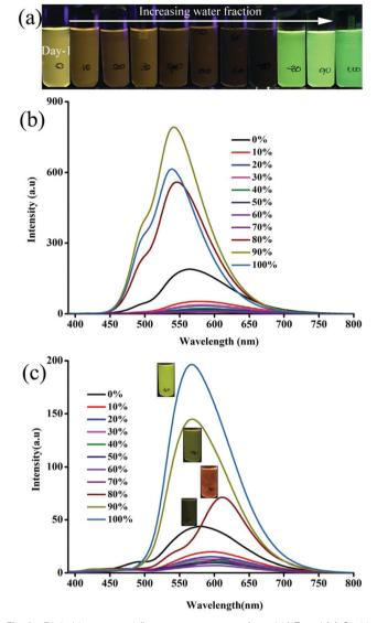
Fig. 1 Digital images and fluorescence spectra (a and b) 3 and (c) 6 with increasing water fraction in a CH<sub>3</sub>CN:water mixture.  $\lambda_{\text{exc}}$  = 365 nm (for the digital images) and 370 nm (for the spectra).
