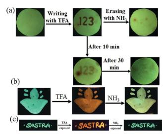
**Fig. 9** Fabricating rewritable/self-erasable fluorescent platforms using **3**-PMMA on (a) a filter paper, (b) symbol on a glass plate and (c) word writing on a glass plate ( $\lambda_{\text{exc}} = 365 \text{ nm}$ ).
