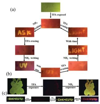
**Fig. 10** Fabricating rewritable/self-erasable fluorescent platforms using **6**-PMMA on (a) a filter paper, (b) a symbol on glass plate and (c) word writing on a glass plate ( $\lambda_{\text{exc}} = 365 \text{ nm}$ ).
