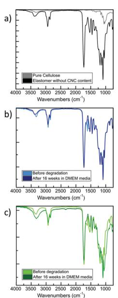
Fig. 4 FT-IR spectra for: (a) pure elastomer and neat CNCs; (b) 6A-PCL-LCE matrix containing 5 wt% CNC before and after 16 weeks in vitro degradation; (c) 6A-PCL-LCE matrix containing 40 wt% CNC before and after 16 weeks in vitro degradation.
