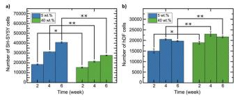
Fig. 8 MTT measurements of (a) SH-SY5Y and (b) hDF cell proliferation within the different composites, 5 wt% and 40 wt%. The error bars represent SEM of the triplicate measurements and \* $p \le 0.05$  and \*\*  $p \le 0.01$ .
