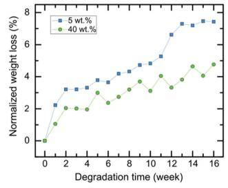
**Fig. 2** Normalized degradation curves of 6A-PLC/CNC nanocomposite scaffolds in DMEM media for 5 wt% (blue curve) and 40 wt% CNCs (green curve).
