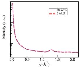
**Fig. 5** X-Ray scattering data from 6A-PCL matrices containing 0 wt% CNC (grey dashed curve) and 50 wt% CNC (black dashed curve), showing a broad halo indicative of the materials being amorphous.
