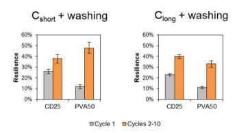
Fig. 7 Energy recovery after the first cycle and mean energy recovery during cycles 2 to 10. The given value is the average value for 3 samples with the standard deviation.
