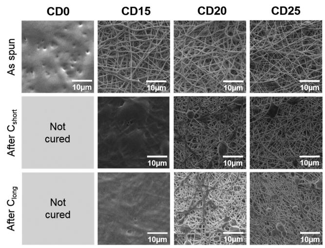
Fig. 2 Influence of the proportion of HPβCD on the PGS/HPβCD/PVP fiber morphology before and after curing for various formulations. CD0 contains 50% of PGS and 50% of PVP; CD15 contains 50% of PGS, 15% of HPβCD and 35% of PVP; CD20 contains 50% of PGS, 20% of HPβCD and 30% of PVP. The morphology is shown after the following curing steps: 24 h at 120 °C followed by 48 h at 140 °C ( $C_{short}$ ) or 24 h at 120 °C, 48 h at 140 °C and 24 h at 170 °C ( $C_{long}$ ).
