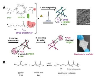
Fig. 1 Strategy for the elaboration of the elastomeric PGS-based fibers. During thermal treatment, pPGS is crosslinked and reaction of -OH groups of HPβCD with -COOH groups of pPGS (in red) occurs (A). Chemical scheme of pPGS synthesis by polycondensation of glycerol and sebacic acid (B).
