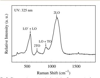
Fig. 5 The room-temperature backscattering Raman spectra from a 325 nm excitation source.  $LO' + LO (430-635 \text{ cm}^{-1})$ , 2TO (720 cm<sup>-1</sup>),  $LO + TO (850-940 \text{ cm}^{-1}) \text{ and } 2LO (1120 \text{ cm}^{-1}).$
