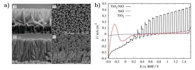
Fig. 6 (a) FE-SEM images of  $TiO_2$  nanorods and  $TiO_2$  nanorods coated with 600 Ni(Cp) $_2$  PEALD cycles. (i) and (ii) show the  $TiO_2$  nanorods and (iii) and (iv) show the nanorods after coating with 20 nm of NiO. (b) j-V curves measured in 1 M KOH (pH = 13.6) of pristine TiO<sub>2</sub>, pristine NiO and TiO<sub>2</sub>–NiO samples. All measurements were performed under 1 sun chopped (AM 1.5G, 100 mW cm<sup>-2</sup>) back-side illumination.
