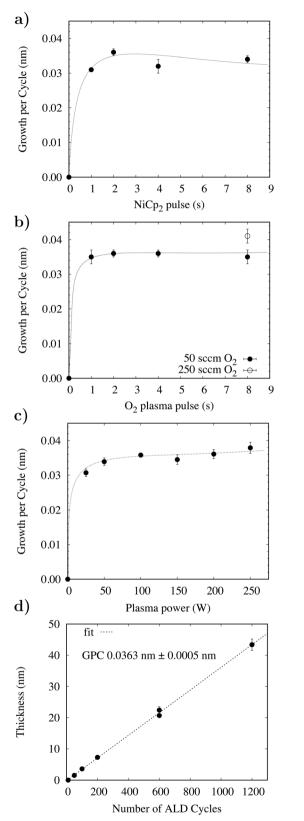
Fig. 2 Optimisation of the Ni(Cp)<sub>2</sub> PEALD process, all depositions completed at 250 °C. (a) Growth rate with respect to the Ni(Cp)<sub>2</sub> delivery pulse. (b) Growth rate vs.  $O_2$  plasma pulse. (c) Growth rate as a function of plasma power. (d) Linearity of growth rate of NiO with respect to the number of ALD cycles.
