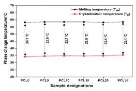
Fig. 9 The phase change temperatures ( $T_{\rm m}$  and  $T_{\rm c}$ ) and the degree of supercooling of neat PCL (PCL0) and its biocomposites with bamboo-root flour
