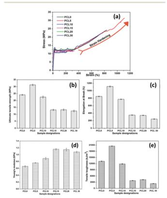
Fig. 3 (a) Representative stress-strain plots, and bar diagrams of the (b) UTS (MPa), (c) % EB, (d) Young's modulus, and (e) tensile toughness of neat PCL (PCL0) and its biocomposites
