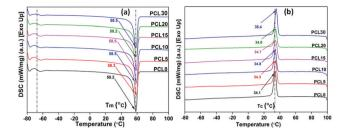
Fig. 8 Representative (a) second heating and (b) first cooling thermograms of melt processed neat PCL and its bamboo-root flour biocomposites.
