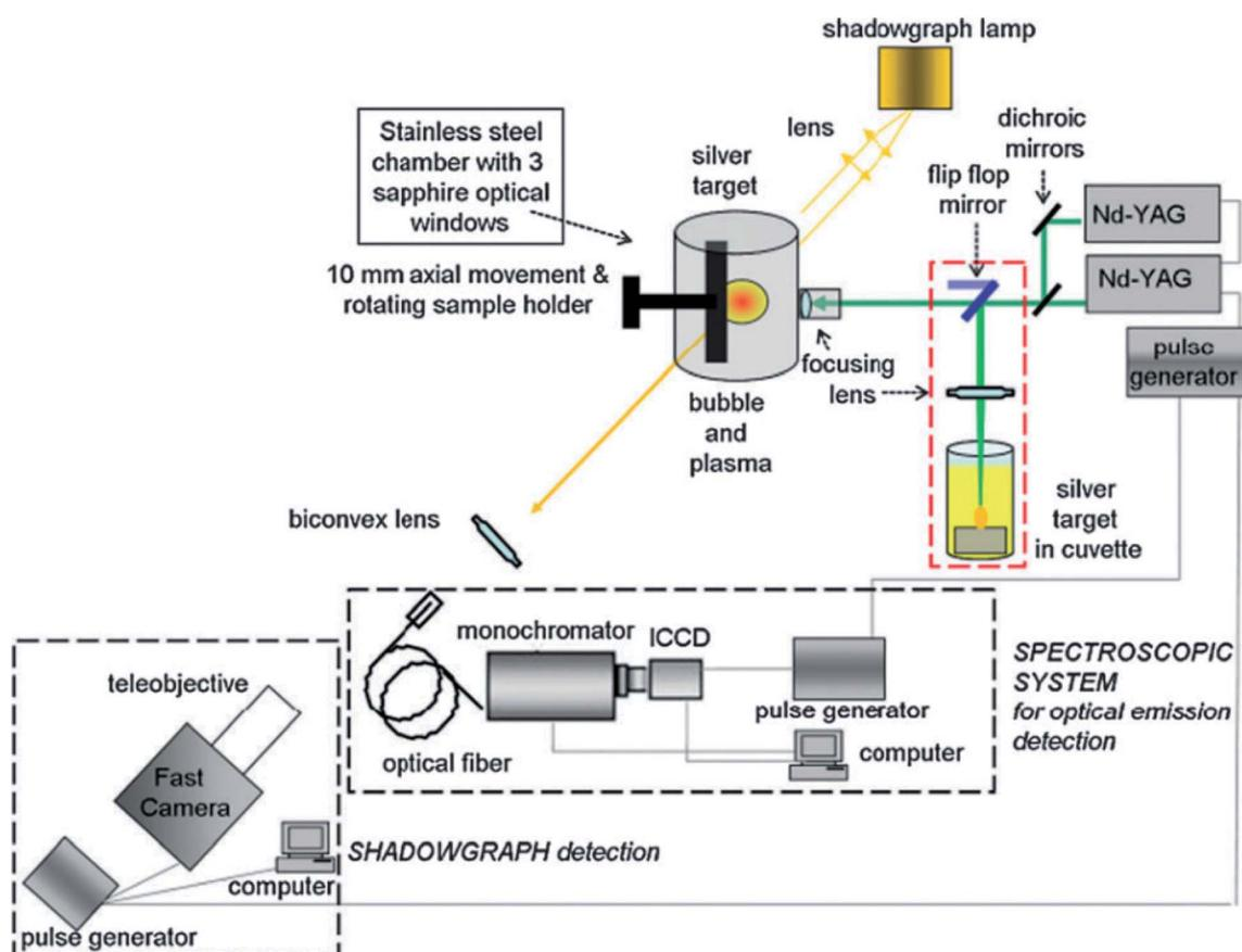
Fig. 3 Schematic of the experimental setup for the OES-based monitoring of NP generation by pulsed laser ablation in gas and liquid.<sup>114</sup>
