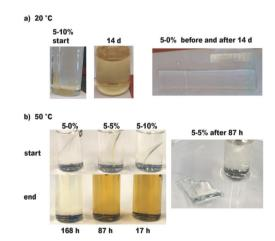
Fig. 6 PU samples before and after degradation test in 5 M HCl in 8:2 (v/v) ethanol: H2O. (a) Room temperature (b) 50 °C.
