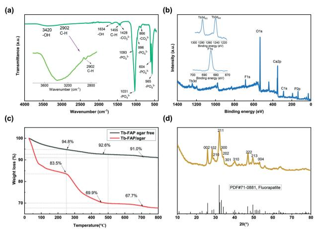
Fig. 1 (a) The FT-IR spectrum of the Tb-FAP/agar nanocomposite. (b) Survey scan of the XPS spectrum of the Tb-FAP/agar nanocomposite with the detailed scans for F 1s and Tb 3d as insets. (c) The TGA plots of the Tb-FAP/agar and Tb-FAP agar free nanocomposite samples. (d) XRD pattern of the Tb-FAP/agar nanocomposite.
