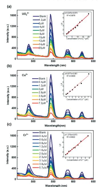
Fig. 3 The concentration effect of (a)  $UO_2^{2+}$ , (b)  $Cu^{2+}$ , and (c)  $Cr^{3+}$ ions on the PL intensity of Tb-FAP/agar ( $\lambda_{\rm ex}$  = 377 nm). Insets show the corresponding fitting curves of the PL intensity of Tb-FAP/agar at 543 nm with the concentration of (a)  $UO_2^{2+}$ , (b)  $Cu^{2+}$ , and (c)  $Cr^{3+}$  ions.
