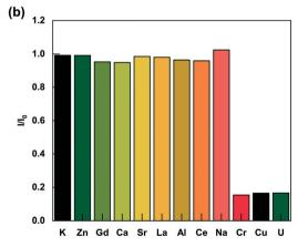
Fig. 2 (a) The emission spectra of the Tb-FAP/agar, Tb-FAP agar free, and Tb-HAP/agar samples. (b) Luminescence intensity of the  $^5D_4 \rightarrow ^7F_5$ transitions (543 nm) of the Tb-FAP/agar (2.5 mL) with different metal ions (10  $\mu$ L, 0.01 M).
