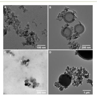
Fig. 1 TEM images of  $nTiO_2$  utilised in experimental work; A research-grade  $nTiO_2$  purchased from Sigma Aldrich; B -  $nTiO_2$  extracted from Skinceuticals<sup>TM</sup> sunscreen (S1); C -  $nTiO_2$  extracted from Boots Soltan<sup>TM</sup> sunscreen (S2); D -  $nTiO_2$  extracted from The Body Shop<sup>TM</sup> liquid foundation (P1).
