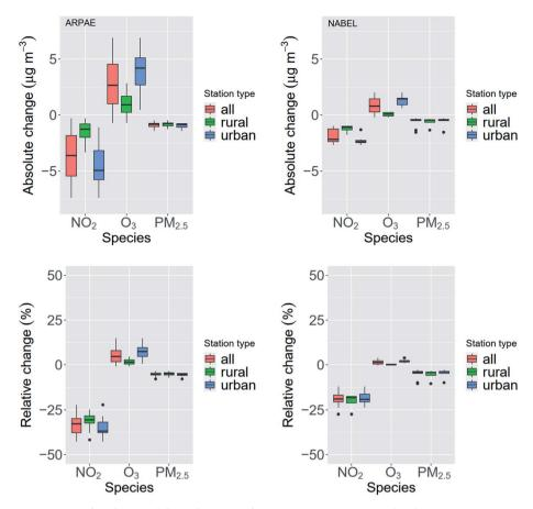
Fig. 3 Boxplots of absolute changes (i.e. CAMx-LOCK - CAMx-BAU) and relative changes in NO<sub>2</sub>, O<sub>3</sub> and PM<sub>2.5</sub> concentrations at all, rural and urban sites. ARPAE network, left panels, and NABEL network, right panels (8 March - 27 April 2020).
