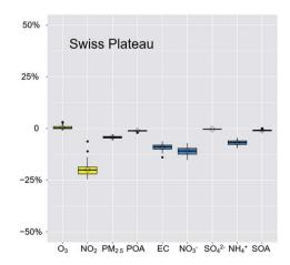
Fig. 5 Relative differences in  $NO_2$ ,  $PM_{2.5}$ , POA, EC,  $NO_3^-$ ,  $SO_4^{2-}$ ,  $NH_4^+$  and SOA concentrations between the CAMx-COVID and the CAMx-BAU scenarios. Po Valley, left panel, and Swiss Plateau, right panel (see Fig. S2† for the details on the regions). The  $PM_{2.5}$  also includes crustal materials (not altered in the CAMx-COVID scenario).
