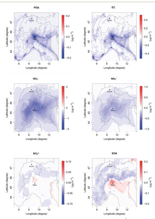
Fig. 6 Absolute changes (i.e. CAMx-LOCK – CAMx-BAU) concentrations of POA, EC, NO<sub>3</sub><sup>-</sup>, NH<sub>4</sub><sup>+</sup>, SO<sub>4</sub><sup>2-</sup> and SOA over the CAMx domain (8 March - 27 April 2020).
