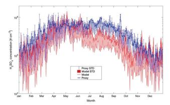
Fig. 13 Yearly mean daily time series of  $\rm H_2SO_4$  concentrations estimated by SOSAA (model) and a proxy parameterization (proxy) at 32.8 m for the years 2007–2018 at SMEAR II. Details of the applied proxy are provided in the text (STD = standard deviation).
