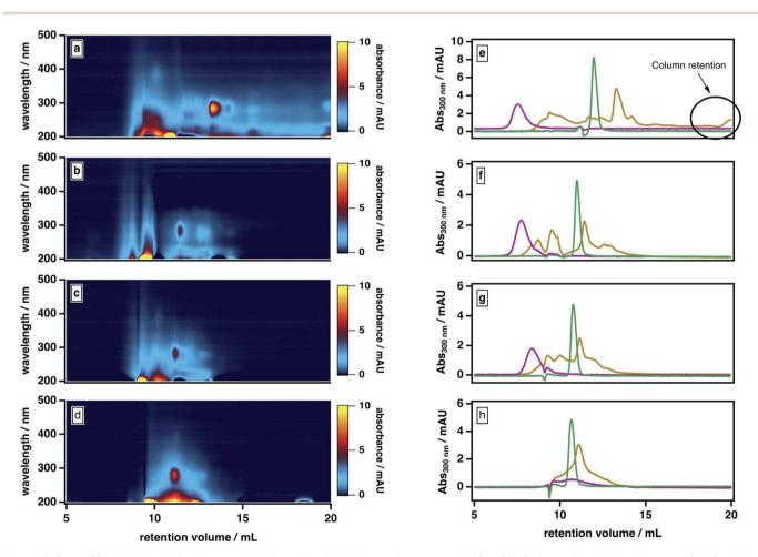
Fig. 4 BrC and SRHA elution behaviour as a function of mobile phase solvent strength: (a-d) BrC absorption density plots and (e-h) singlewavelength (300 nm) chromatograms (— SRHA, — acetone, — BrC). Experiments were conducted under the following mobile phase organic modifier conditions: 25% ACN (a and e), 50% ACN (b and f), 60% ACN (c and q), and 70% ACN (d and h). In all cases, the remainder of the mobile phase was 20 mM phosphate buffer (pH 6.8).
