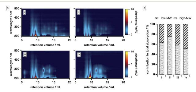
Fig. 3 BrC elution behaviour as a function of mobile phase solvent strength: (a) absorption density plots and (b) absorption contributed by high-MW and low-MW BrC fractions, with the latter calculated as described in the ESI.† Experiments were conducted under the following mobile phase organic modifier conditions: (i) 50% MeOH/0% ACN, (ii) 40% MeOH/10% ACN, (iii) 25% MeOH/25% ACN, (iv) 0% MeOH/50% ACN. In all cases, the remainder of the mobile phase was 20 mM phosphate buffer (pH 6.8).
