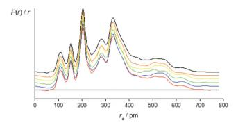
Fig. 3 Experimental (black) and theoretical [+77++ (red), +143--(blue), -91-(-) (green), +165+- (yellow), +51-- (orange)] radial distribution curves, P(r)/r, for 1. Traces are offset for clarity. Before Fourier inversion the data were multiplied by  $s \exp(-0.0020s^2)/(Z_{CL} - f_{CL})/(Z_{CL} - f_{CL})$
