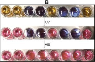
Fig. 5 Binary models for applying 2NB-RZ (dark yellow plates) and RZ (blue plates) in information encryption using UV (365 nm) and VIS (525 nm) as password entries
