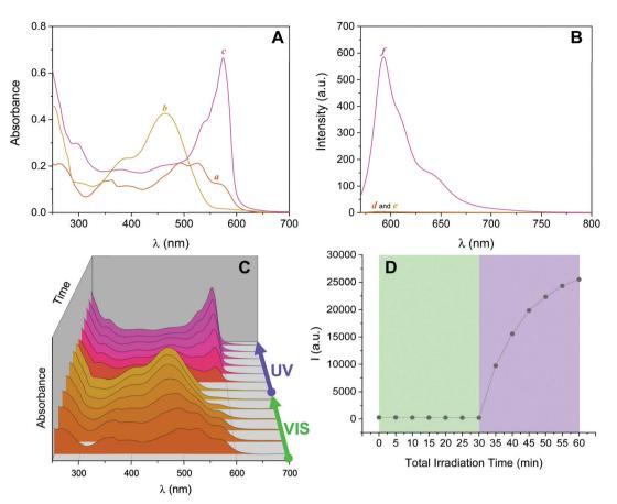
Fig. 3 Top panels: Absorption (panel A) and emission (panel B,  $\lambda_{Ex}$  = 550 nm) spectra of a solution of **2NB-RZ** (18  $\mu$ M, 20 °C, CH<sub>3</sub>OH, NH<sub>2</sub>OH 3000 eq.) before irradiation (a and d), after irradiation at 525 nm (b and e, 30 min) and after additional irradiation at 365 nm (c and f, 30 min). Bottom panels: Evolution of the absorbance (panel C) and integrated emission intensity (panel D) during the illumination cycles.
