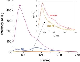
Fig. 1 Absorption (top panel) and emission (bottom panel,  $\lambda_{Ex}$  = 550 nm) spectra of RZ, RF, 2NB-RZ and 2NB-RF (18 μM). Spectra were recorded at 20 °C in  $H_2O$  (RZ and RF) or  $CH_3OH$  (2NB-RZ and 2NB-RF) in the presence of NH2OH (excess, 3000 eq.).
