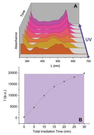
Fig. 4 Evolution of the absorbance (top panel) and integrated emission intensity (bottom panel,  $\lambda_{Ex}$  = 550 nm) of a solution of **2NB-RZ** (18  $\mu$ M, 20 °C, CH<sub>3</sub>OH, NH<sub>2</sub>OH 3000 eq.) before and after irradiation at 365 nm (0-30 min. 5 min irradiation intervals)
