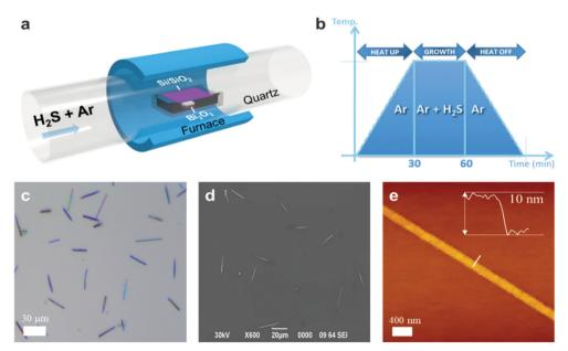
Fig. 1 The synthesis method of  $Bi_2S_3$  and its characterization. (a) Schematic illustration of experimental set-up of  $Bi_2S_3$ , (b) diagram of synthesis process of Bi<sub>2</sub>S<sub>3</sub>, (c) OM image of as-grown Bi<sub>2</sub>S<sub>3</sub>, (d) SEM image of as-grown Bi<sub>2</sub>S<sub>3</sub>, and (e) AFM image and height profile of as-grown Bi<sub>2</sub>S<sub>3</sub>.
