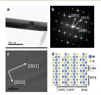
Fig. 4 Structure analysis of Bi<sub>2</sub>S<sub>3</sub>. (a) TEM image of Bi<sub>2</sub>S<sub>3</sub> on a TEM grid, (b) SAED patterns of single crystalline Bi<sub>2</sub>S<sub>3</sub>, (c) HRTEM image of anisotropic Bi<sub>2</sub>S<sub>3</sub> structure, and (d) schematic illustration of Bi<sub>2</sub>S<sub>3</sub> crystal structure.
