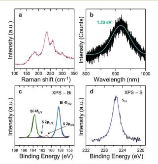
Fig. 2 Characterization of optical properties and stoichiometry analysis of Bi<sub>2</sub>S<sub>3</sub> (a) Raman spectrum of Bi<sub>2</sub>S<sub>3</sub>, (b) PL spectrum of Bi<sub>2</sub>S<sub>3</sub>, (c) XPS spectrum of Bi 4f peaks and S 2p peaks, and (d) XPS spectrum of S 2s
