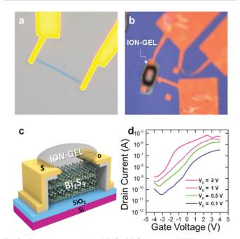
Fig. 5 Electronic properties of Bi<sub>2</sub>S<sub>3</sub>: (a) OM image of FET based on asgrown Bi<sub>2</sub>S<sub>3</sub>, (b) OM image of the ion-gel gated transistor of Bi<sub>2</sub>S<sub>3</sub>, (c) schematic diagram of ion-gel gated Bi<sub>2</sub>S<sub>3</sub> FET, (d) transfer characteristics of Bi<sub>2</sub>S<sub>3</sub> transistor.
