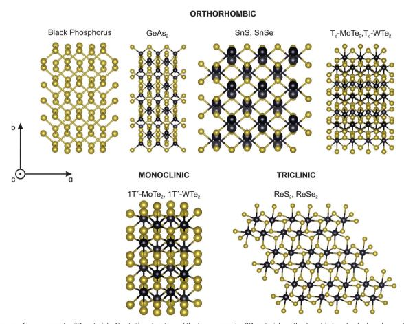
Fig. 3 Classes of low-symmetry 2D materials. Crystalline structure of the low-symmetry 2D materials: orthorhombic (e.g. back phosphorus, GeAs<sub>2</sub>, SnS, SnSe, T<sub>d</sub>-MoTe<sub>2</sub>, T<sub>d</sub>-WTe<sub>2</sub>), monoclinic (e.g. 1T'-MoTe<sub>2</sub>, 1T'-WTe<sub>2</sub>) and triclinic (ReS<sub>2</sub>, ReSe<sub>2</sub>).
