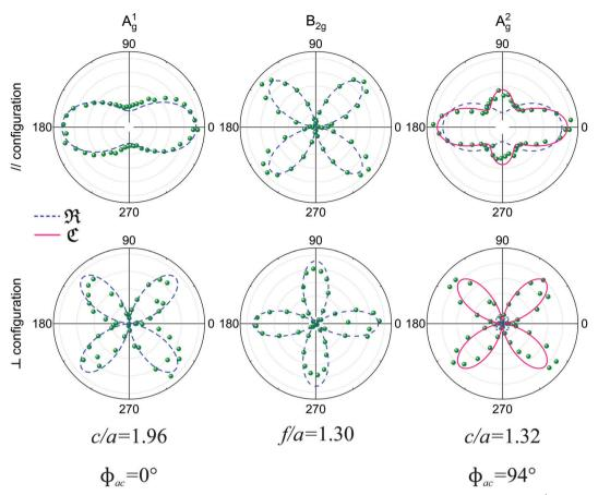
Fig. 5 Angle-resolved Raman response of the orthorhombic black phosphorus. Angular dependence of the intensities of the  $A_q^1$ ,  $B_{2q}$  and  $A_q^2$  modes in the parallel (||, top panel) and crossed (\perp , bottom panel) polarization configurations for an exfoliated BP flake for an excitation energy of 2.33 eV. The corresponding tensor element ratios and phase differences extracted from the fitting process are also shown. Adapted with permission from ref. 21.
