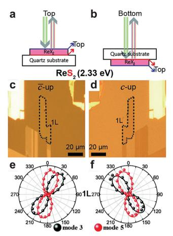
Fig. 9 The flipping-like a coin behavior in triclinic 2D materials. Scheme of the laser beam to probe the vertical orientation in triclinic  $ReX_2$  (X = S or Se) in the (a) "up" and (b) "down" sample's orientation. Optical images of the monolayer  $ReS_2$  in the (c) "up" and (d) "down" orientation show in (a and b). Angle-polarized Raman response of modes 3 and 5 of monolayer  $ReS_2$  in the (e) "up" and (f) "down" orientations. Adapted with permission from ref. 51.
