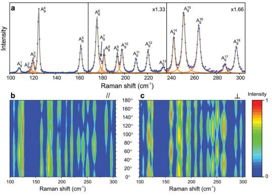
Fig. 7 Characteristic Raman spectrum of the triclinic ReSe<sub>2</sub>; (a) Raman spectrum of a monolayer ReSe<sub>2</sub> showing the 18 A<sub>a</sub> modes predicted by group theory. Typical angle-resolved Raman map of ReSe<sub>2</sub> in the (b) parallel (||) and (c) crossed (\(\perp\)) configurations. The spectra and mapping were collected with a 2.33 eV laser energy. Adapted with permission from ref. 19.
