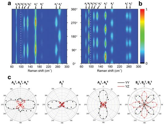
Fig. 6 Typical angle-resolved Raman map of a monoclinic 1T'-MoTe<sub>2</sub>. Raman map in the (a) parallel ( $\parallel$ ) and (b) crossed ( $\perp$ ) polarization configurations. (c) Angular dependence of the intensities of the 1T'-MoTe<sub>2</sub> peaks shown in (a) and (b). The angle-resolved Raman map was constructed using two excitation energies: 1.96 eV (below 100 cm<sup>-1</sup>) and 2.33 nm (above 100 cm<sup>-1</sup>). Adapted with permission from ref. 50
