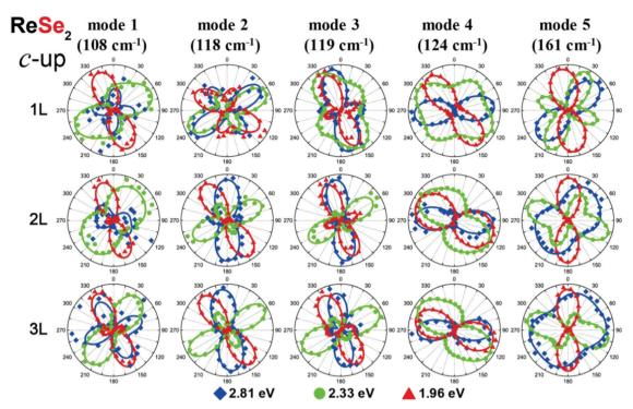
Fig. 11 Resonant Raman response of a triclinic ReSe<sub>2</sub>. Resonant angle-resolved Raman dependence of some modes of a few-layered ReSe<sub>2</sub> in the "up" orientation for excitation energies of 1.96, 2.33, and 2.81 eV, respectively. Adapted with permission from ref. 51.
