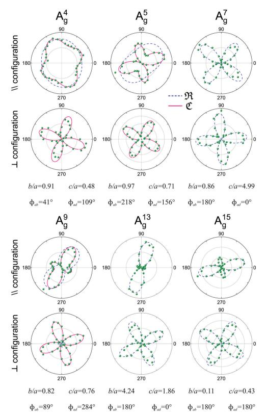
$\textbf{Fig. 8} \quad \textbf{Typical Raman polar plots of a monolayer triclinic } \textbf{ReSe}_2. \ \textbf{Angular dependence of the intensities of 6} \ \textbf{A}_g \ \textbf{modes in the parallel (} \parallel \textbf{)}$ and crossed (1) configurations for an exfoliated monolayer ReSe2 collected using an excitation energy of 2.33 eV. The corresponding tensor element ratios and phase differences extracted from the fitting process are also shown. Adapted with permission from ref. 19.
