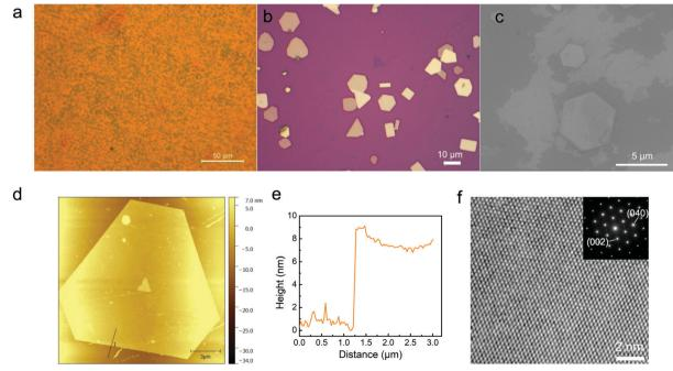
Fig. 1 (a) Optical image of graphene-Mo<sub>2</sub>C grown on a Cu foil. (b) Optical image of graphene-Mo<sub>2</sub>C after transferred to the Si/SiO<sub>2</sub> substrate. (c) SEM image of the graphene-Mo<sub>2</sub>C heterostructure. (d) AFM topography of the graphene-Mo<sub>2</sub>C heterostructure. (e) AFM cross-setional profile along the black line in (d). (f) HRTEM image of Mo<sub>2</sub>C showing the atomic structure. The inset shows the SAED result.
