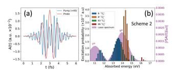
Fig. 5 (a) Vector potential A(t) for an attosecond pulse train after applying a frequency filter (blue), and the probe pulse with a frequency of the 3rd harmonic of the generating 800 nm IR field (red). (b) Excitation probabilities for the  ${}^{1}\Sigma_{u}^{+}$  electronic states for the filtered pulse.
