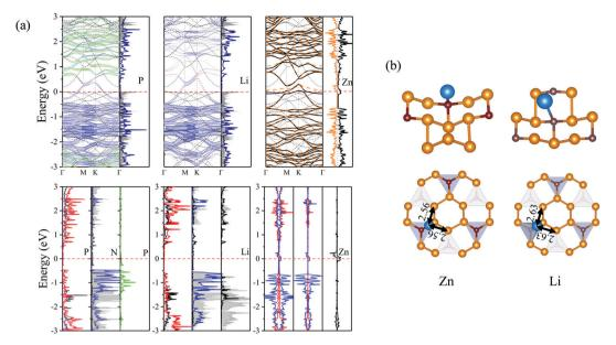
Fig. 10 (a) Orbital resolved band structure, DOS and PDOS of their system with substrate adsorbed P, Li and Zn adatoms, respectively. The zero of energy is set to  $E_f$ , shown by the red dashed-dotted line. (b) Schematic view of the most stable site and relative position parameters of adatoms for adsorption of Zn and Li on  $N_2P_6$ .
