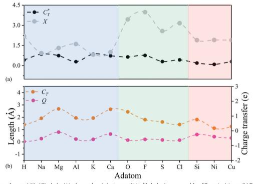
Fig. 4 (a) Charge transfer capability ( $C_T^*$ , dashed black curve) and electronegativity (X, dashed grey curve) for different adatoms. (b) Comparison between the distortion magnitude of  $N_2P_6$  structure (Q, dashed rose curve) and the charge transfer of adatoms ( $C_T$ , dashed orange curve). The adsorption type of T<sub>N</sub>, T<sub>P</sub>, H<sub>PP</sub> are represented by light blue, green and red area, respectively.
