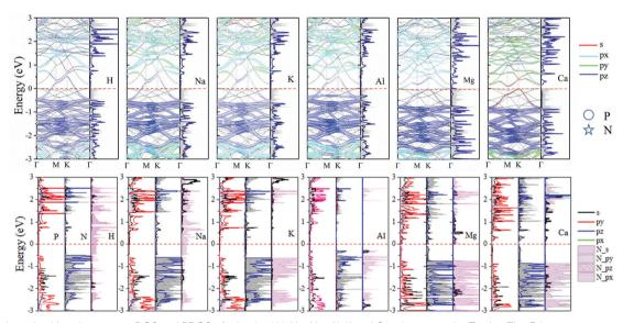
Fig. 6 Orbital resolved band structure, DOS and PDOS of adsorbed H, Na, Mg, Al, K and Ca adatoms at the  $T_N$  site. The  $E_f$  is set to zero as shown by the red dashed-dotted line
