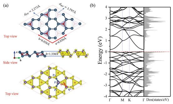
Fig. 1 (a) The top and side view of optimized structure, total charge density of  $N_2P_6$  monolayer. Rufous (cyan), or red (brown) dots are N (P) atoms. (b) The band structure and density of states (DOS) of N<sub>2</sub>P<sub>6</sub> corresponding to the left structure.
